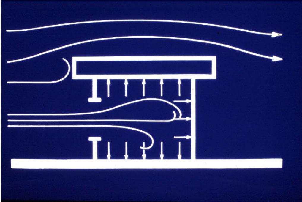
**Figure 1. Simplified schematic showing the airflow (long arrows) extending over and into a building with a windward wall opening. The wind pressure on the building's interior actually increases, resulting in additional uplift or outward forces (small arrows). Thus, opening windows when a tornado approaches could actually be detrimental to the structure. Figure courtesy of IDR at Texas Tech University.**
