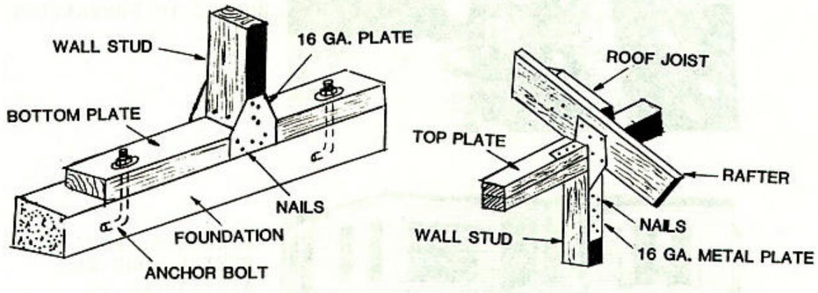
**Figure 5. Recommended connection details to resist wind uplift: a) wall-foundation detail, and b) roof-wall detail.**
